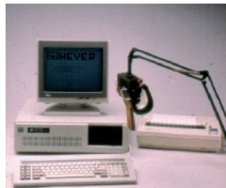
Figure 6. Carima System (1989). The first PC-controlled rhinomanometer in the world, produced by Heyer, Bad Ems, Germany. Due to a still existing problem of sensor relocation sensitivity, the case is vertically mounted onto a stand.
